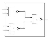
G1, G2 & G3 are the component label for the current instantiation of the nandg component. The ordering of the actual is not important. Here S1 is actual and Y is the formal.
