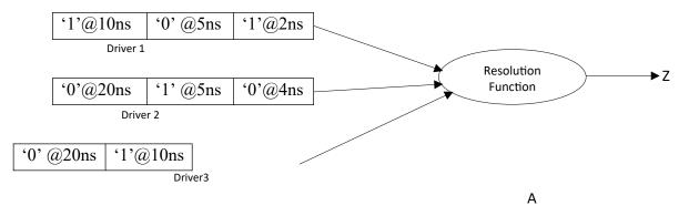
The resolution function is associated with the signal by specifying the name in the signal declaration. (signal declaration could wired-or, wired and, average value etc.,) considering the wired-OR operation for the above example, the correct way if representing it is
