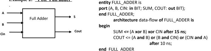
Two signal assignment statements are used to represent the dataflow of the FULL\_ADDER entity. Whenever an event occurs on signals A, B, or CIN, expressions of both the statements are evaluated and the value to SUM is scheduled to appear after 15 ns while the value to COUT is scheduled to appear after 10 ns. The after clause models the delay of the logic represented by the expression.
