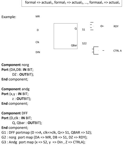
In this case considering G2, MR is an actual which is declared in the entity port list is associated with the first port (port DA, a formal) of the norg gate, signal ready is associated with the third port (DZ) and S1 is associated with the second port (DB of norg gate.)
