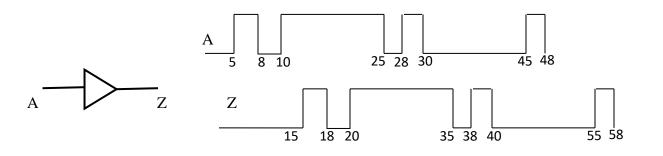
In this case, spikes would be propagated through instead of being ignored as in the inertial delay case.
